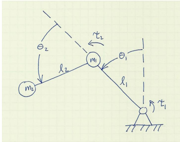
Figure 1: RR Arm: A planar arm with two point-masses and two revolute joints.
